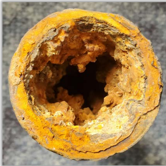
Corroded & Aging Smithville Waterline Segments
